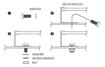
Figure 5. Mounting using bolts on the transversal bars.
