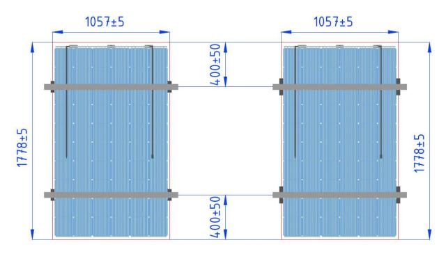
Figure 2. 6.3 SOLID Pro P(M).60 mounting with four fixing points and transversal rails.
