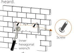
b) Insert expansion bolt into the hole, use rubber hammer to knock the expansion screw bolt into the wall.
