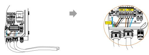
4) Pass the battery power wire through the BAT port of The X3-Matebox advanced, then find the BAT+ and BAT- ports in the X3-Matebox advanced, insert each wire accordingly, and use the screwdriver to lock the screws.
