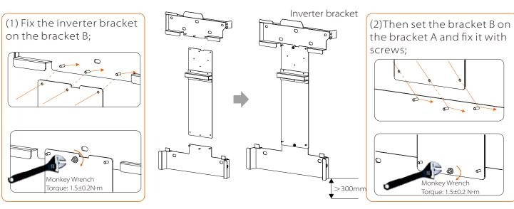
Note: When installing the bracket, be sure to use a spirit level to test and keep the bracket parallel to the horizontal plane.
