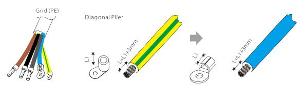
3) Pass the Grid/Load line through the Grid/Load port of the X3-Matebox advanced, then find the Grid(R/S/T/N) port and Load (R/S/T/N) ports in the X3-Matebox advanced, insert each line, and use the screwdriver to lock the screws.
