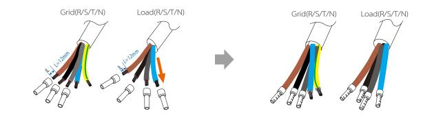
b) Grid(PE) strip the grounding cable insulation(length"L"), insert the stripped cable into the R type terminal, and then clamp it.
