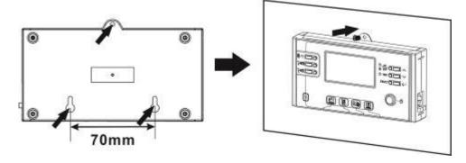
**Note:** Installation to the wall should be implemented with the proper screws. Refer chart for recommended spec of screws.
