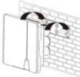
Fig. 6: Mounting the inverter to the wall bracket
