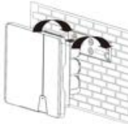
Sl. 6: Razsmernik vpnite v stenski nosilec.
